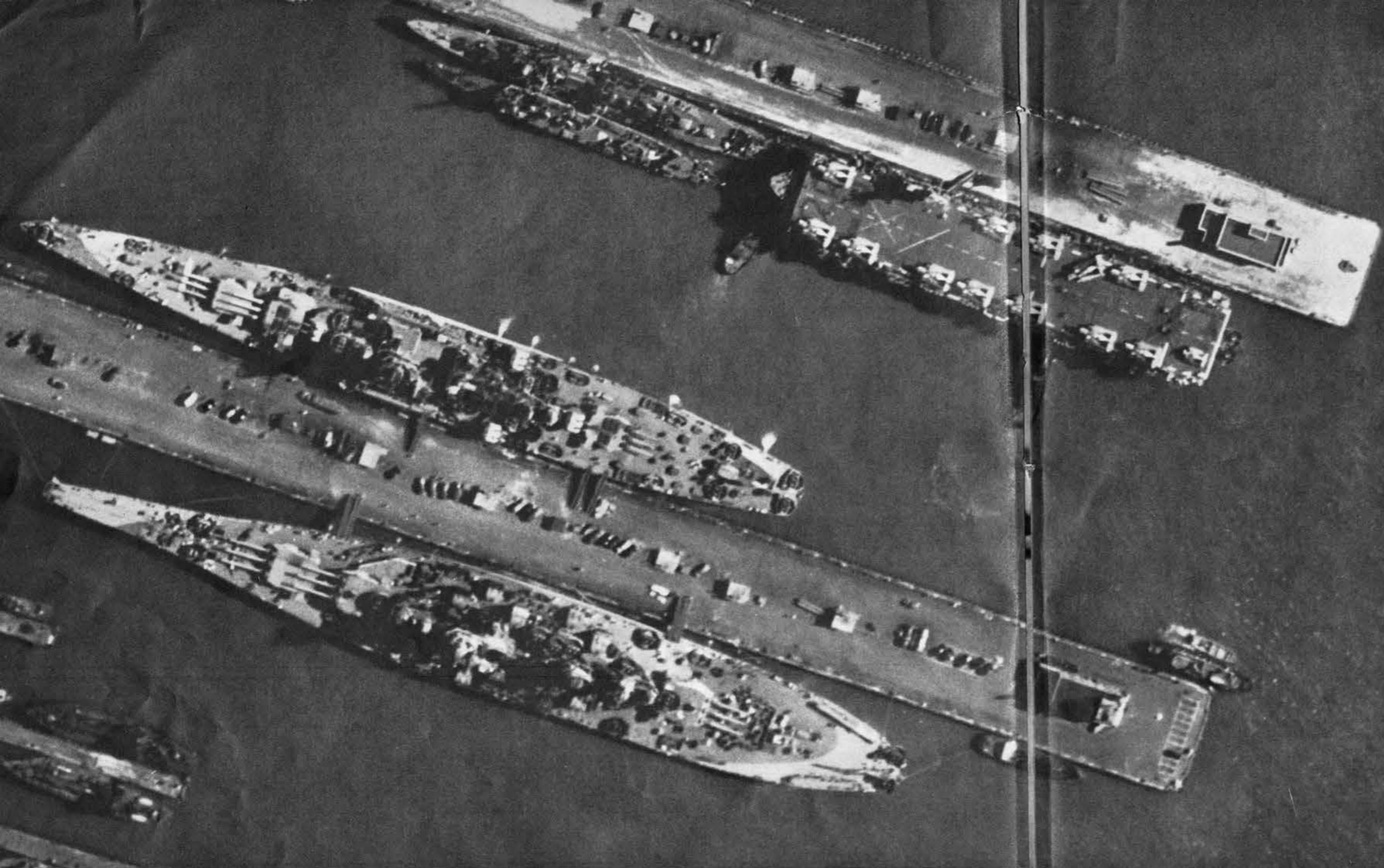
IOWA SHOWS LONG FORWARD TAPER, ROUNDED STERN OF MODERN BB. ALTHOUGH OVERSIZE, ALASKA (ABOVE) HAS GRACEFUL LINES OF CRUISER. NOTE
